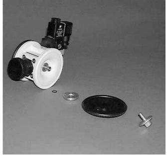
Inspection of diaphragms, pistons, disc spring and shaft is now possible.
