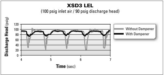
These charts show discharge head fluctuations for a diaphragm pump with and without a dampener. By reviewing the variation in pressure, the level of dampening can be estimated for an application. For example, the head pressure generated by a 3" pump operating at 100 psig air inlet pressure and 90 psig head pressure varies between 21 psig and 103 psig resulting
