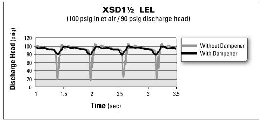
These charts show discharge head fluctuations for a diaphragm pump with and without a dampener. By reviewing the variation in pressure, the level of dampening can be estimated for an application. For example, the head pressure generated by a 1-1/2" pump operating at 100 psig air inlet pressure and 90 psig head pressure varies between 12 psig and 108
