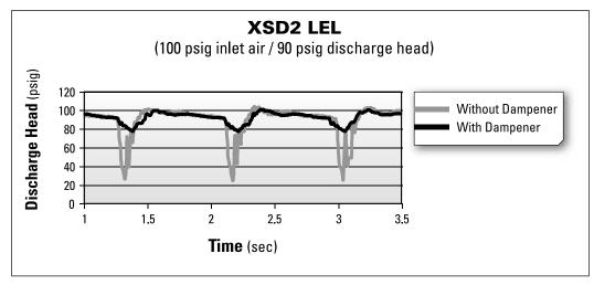
These charts show discharge head fluctuations for a diaphragm pump with and without a dampener. By reviewing the variation in pressure, the level of dampening can be estimated for an application. For example, the head pressure generated by a 2" pump operating at 100 psig air inlet pressure and 90 psig head pressure varies between 20 psig and 102 psig resulting
