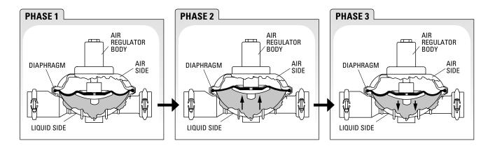
A compressed air line attached to the air regulator body sets and maintains pressure on the air side of the diaphragm. As the reciprocating pump begins its stroke, liquid discharge pressure increases which flexes the Equalizer® diaphragm inward. This action accumulates fluid in the liquid chamber (see phase 2).
