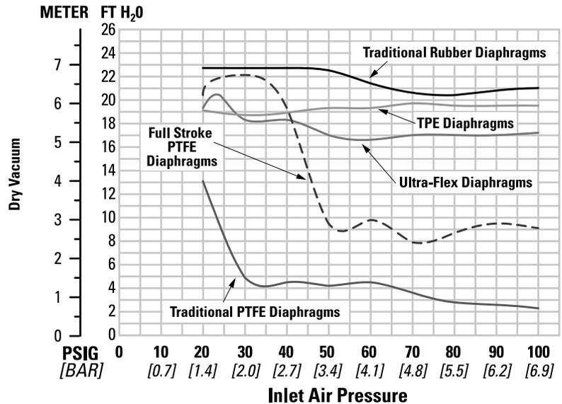
Suction lift curves are calibrated for pumps operating at 305 m (1,000') above sea level. This chart is meant to be a guide only. There are many variables which can affect your pump's operating characteristics. The
