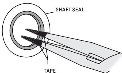
**SHAFT SEAL INSTALLATION:**
