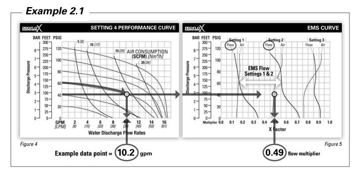
This is an example showing how to determine the inlet air pressure and the EMS setting for your Pro-Flo X™ pump to optimize the pump for a specific application. For this example we will be using an application requirement of 18.9 lpm (5 gpm) flow rate against 2.8 bar (40 psig) discharge pressure. This example will illustrate how to calculate the air consumption that could be expected at this operational point.
