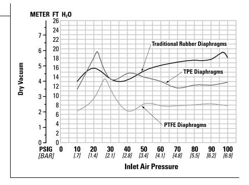
Suction lift curves are calibrated for pumps operating at 305 m (1,000') above sea level. This chart is meant to be a guide only. There are many variables which can affect your pump's operating characteristics. The number of intake and dis-
