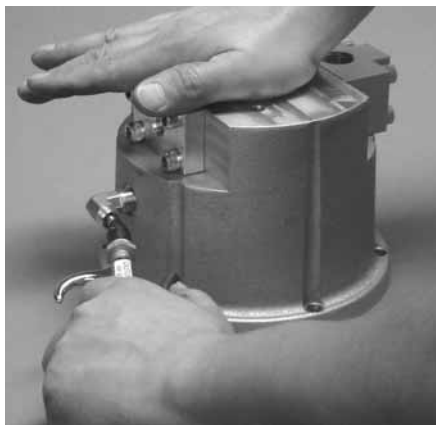
Step 8. Figure 8 To remove the power piston from the liquid chamber, first place the liquid chamber onto a table or sturdy flat surface. Next, with the liquid chamber resting on the bolted flange, apply 1.0 bar (15 psig) of air pressure, via a rubber tipped air nozzle, into the brass elbow located at the same side as the pump discharge port. CAUTION: The power piston may come out of the liquid chamber with considerable force. Altering the disassembly method above is not recommended and may cause physical harm.
