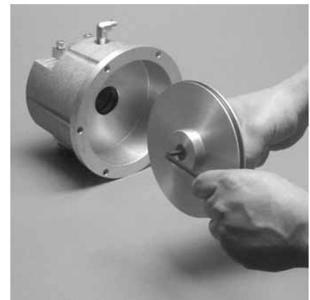
Step 10. Figure 10 Using a 5mm (3/16") hex head wrench, remove the liquid piston from the power piston by turning the power piston screw counter-clockwise.
